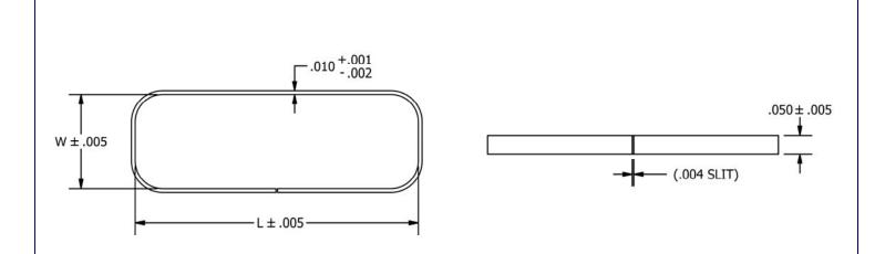
These preforms are designed specifically for SHP HMMHE connectors. They provide optimum flow and fillet when used with the recommended preform well and are available in two solder alloys per EIA J-STD-006: Sn62, Sn63.
